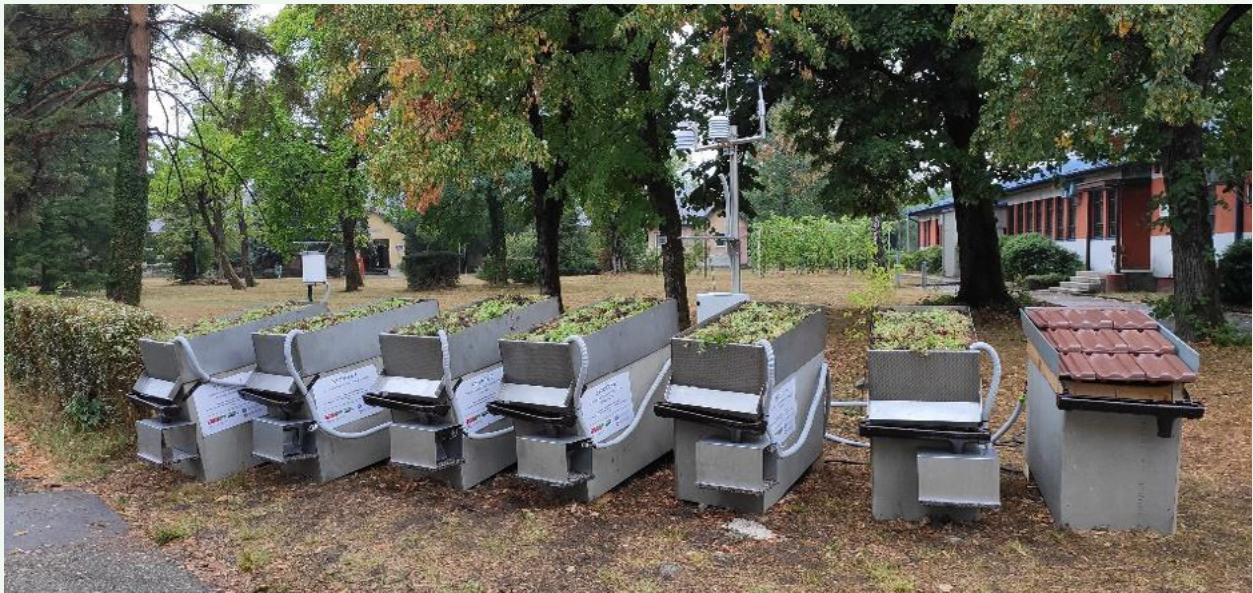
Figure 19. Experimental green roofs in Banja Luka
